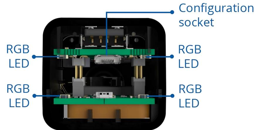
Figure 2 FMP100 device view (Without covers)
