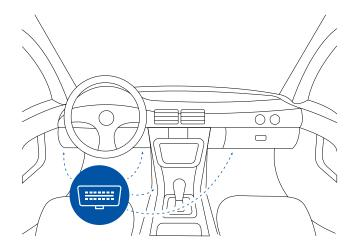
Most common OBDII connector locations.
