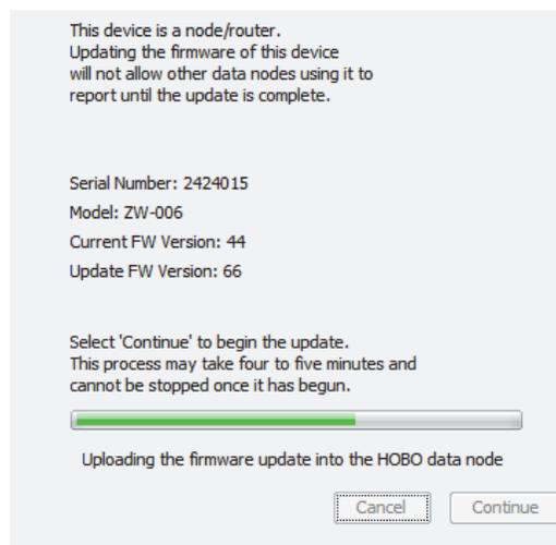
When the firmware is saved to the device, the LED will flash red on the receiver and green on a data node. A message appears at the end when the update is successfully completed.
