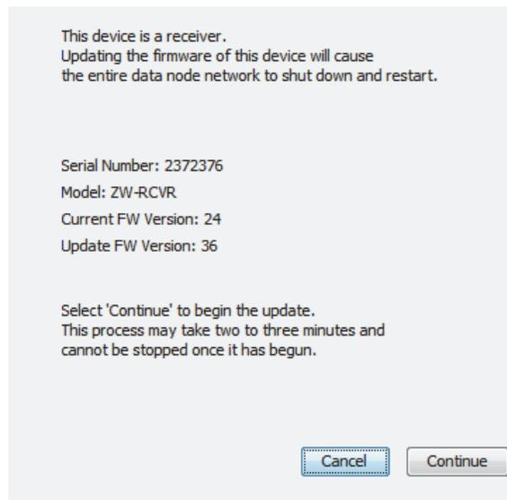
7. The firmware is updated in the device; check the progress on the screen during the update as shown in the following example of a node being updated.
