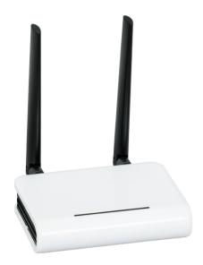
The Efento Gateway automatically transmits data from Efento Bluetooth Low Energy sensors to Efento Cloud or any other IoT platform over a cellular (LTE) network. This gateway enables the creation of remote monitoring systems and is compatible with all types of Efento sensors. Equipped with internal memory, the Efento LTE Gateway buffers sensor data, while its built-in backup battery ensures uninterrupted power during outages. The device is easy to set up in just minutes using a free mobile app.
