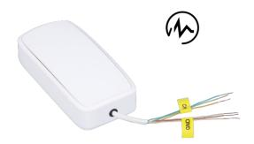
Efento 0-10 V sensor interface allows users to connect any type of analog sensor. Device can be equipped with up to two analog interfaces (2 x 0-10 V). Sensors can be powered either from the device's battery or by an external power source. Data from the analog sensors can be presented as voltage (0-10 V) or converted to other measurement types once it reaches the Efento Cloud platform.
