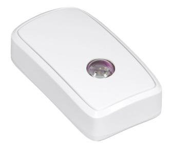
Efento NB-IoT loggers transmit the data over cellular network (Narrowband IoT) and do not require any additional devices (router, gateway, etc.). Sensors are also equipped with Bluetooth Low Energy interface, which allows quick and easy configuration with a smartphone. Efento NB-IoT sensors can be integrated with any cloud platform. You can use a free mobile application to configure the device and read the data from its memory.
