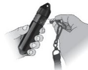
**Important:** When storing or transporting the logger, keep the magnetic fob (or any other magnet) a minimum of 1" away from the logger so that you do not inadvertently drain the logger's battery.
