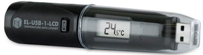
This standalone data logger measures and stores more than 16,000 temperature readings over a -35 to +80°C (-31 to +176°F) range with a resolution of 0.5°C (0.5°F).
