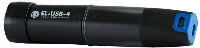
This stand-alone data logger measures and stores over 32,000 current loop readings over a 4-20mA d.c. range at a resolution of 0.05mA d.c.
