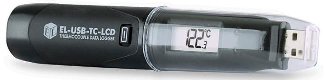
This standalone data logger measures and stores more than 32,000 temperature readings from a J, K or T-type thermocouple at a resolution of 0.5°C (1°F). It comes supplied with a K-type thermocouple capable of measuring from 0 to 200°C (32 to 392°F).
