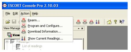
The process of retrieving data stored within an iMiniPlus PDF Logger does not erase it from the memory. If the iMiniPlus is currently recording while you retrieve the information, it will continue to record without interruption. The Download Information feature initiates the Download Wizard.
