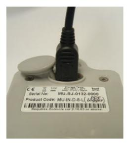
Simply connect the logger to your PC and wait until the Operating System installs device drivers. Please allow Windows sufficient time to install the device. Please do not connect multiple loggers at the same time since it may cause unexpected behaviour.
