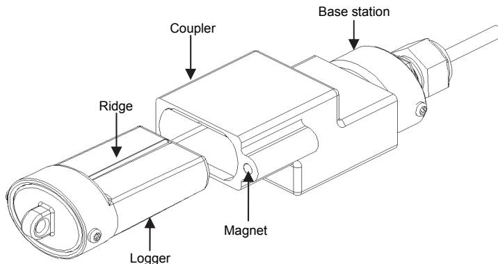
Remove the logger from the coupler when it is not communicating with the computer. Storing the logger in the coupler will cause the battery to run down prematurely.
