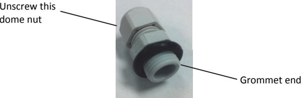
2. Feed the wires on the side of the case through the grommet assembly, O-ring side first. Hand-tighten the grommet end of the assembly in the hole so that the O-ring is snug against the protective case. Feed the wires through the dome nut and then hand-tighten it back on the assembly. Turn an additional quarter-turn with a wrench to further tighten, but do not force.
