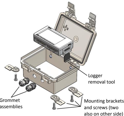
1. Use a Phillips screwdriver to attach the four mounting brackets to the back of the case.
