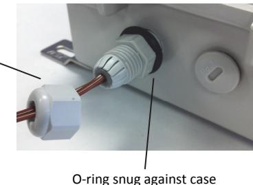
3. Repeat steps 6 and 7 with the other assembly and thermocouples. If there are no thermocouples in the other port, then screw the dome plug into the open port so the O-ring is snug against the case as shown below.
