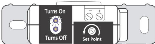
STEP 1: Turn the setpoint screw counter-clockwise until the Status Open LED turns off and the Status Closed LED turns on. (Sensor should be in this state right out of the box.)
