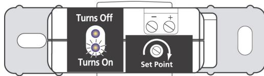
STEP 1: Turn the setpoint screw clockwise until the Status Closed LED turns off and the Status Open LED turns on.
