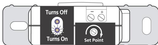
STEP 2: Slowly turn the setpoint screw clockwise until the Status Closed LED turns off and the Status Open LED turns on.
