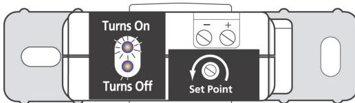
STEP 2: Slowly turn the setpoint screw counter-clockwise until the Status Closed LED turns on and the Status Open LED turns off.
