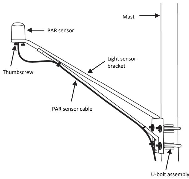
PAR Smart Sensor Bracket Mounting
