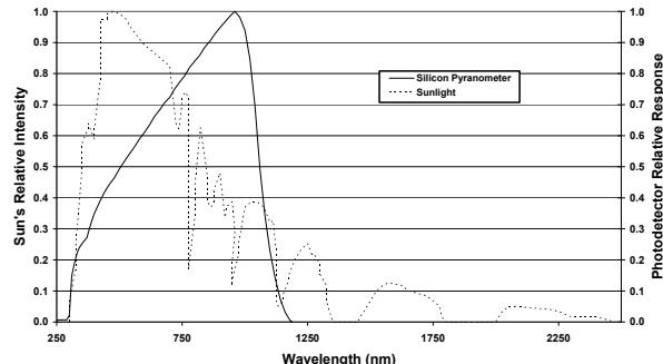
Plot A: S-LIB-M003 Silicon Pyranometer Response Curve
