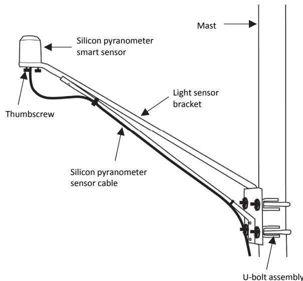
Silicon Pyranometer Sensor Bracket Mounting
