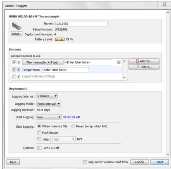
3. **Select the internal 10k thermistor (temperature) channel to log (optional) and type a label if desired.** This internal 10K thermistor measures ambient temperature and is used for cold-junction compensation of the thermocouple output.
