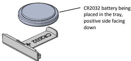
4. With the LCD screen still facing up, slide the tray back into the logger. The LCD should display "HOBO" briefly after correctly installing the battery.
