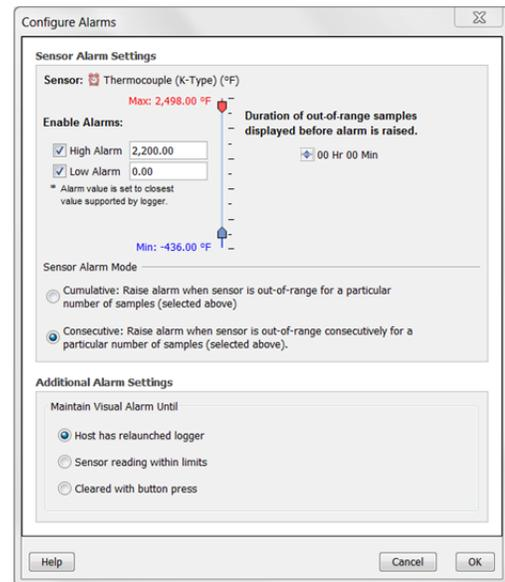
6. Choose how long the logger should maintain the sensor alarm once it has tripped. Select "Host has relaunched logger" if you want the alarm to remain visible on the LCD until the next time you relaunch the logger. Select "Sensor reading within limits" if you want the alarm to clear once the sensor reading returns to the normal range between the high and low alarm limits. Select "Cleared with button press" if you want the alarm to remain on until you press the Alarm/Stats button on the logger.
