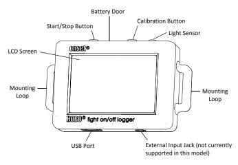
**Start/Stop Button:** Press this button for 3 seconds to start or stop logging data. This requires configuring the logger in HOBOware with a push button start or stop (see *Setting up the Logger*). You can also press this button for 1 second to record an internal event (see *Recording Internal Logger Events*) or to turn the LCD screen on if the option to turn off the LCD has been enabled (see *Setting up the Logger*).
