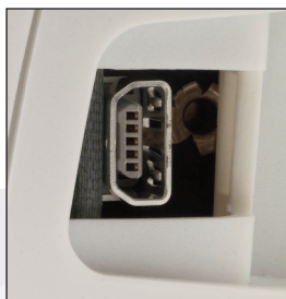
Above: Detail of USB socket
