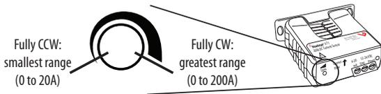
To determine the best amperage range for an application, first set the load to the maximum amperage that will be used. Use the LED as a guide to adjust the potentiometer to its optimum setting. Verify the measured output current matches the load current using a current clamp meter.
